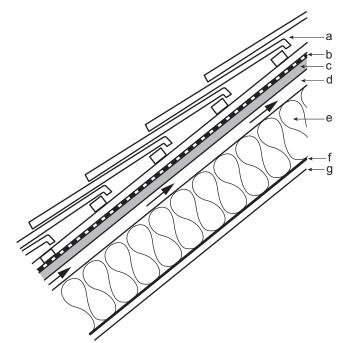
Figure 2.12: Example of a warm roof with sloping ceiling and insulation between rafters. There must be adequate ventilation above the insulation
