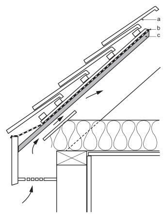
Figure 2.11: Example of a cold roof space with insulation at ceiling level. The roof space must be adequately ventilated a: tiles on battens and counterbattens b: tiling underlay
